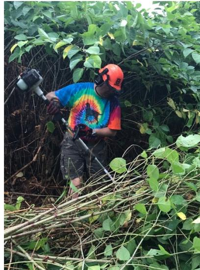
Singular-bladed brush cutter makes a clean cut on large stems. Do NOT weed whack! July 2020
